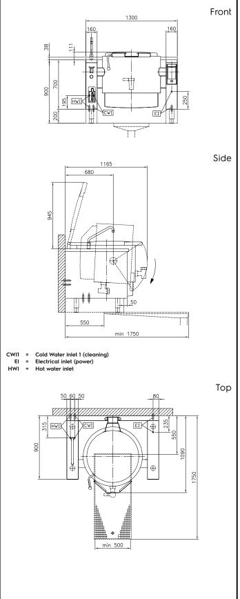
ProThermetic Sprint Electric Tilting Boiling Pan, 150lt Hygienic Profile, Freestanding with Stirrer The company reserves the right to make modifications to the products without prior notice. All information correct at time of printing.
